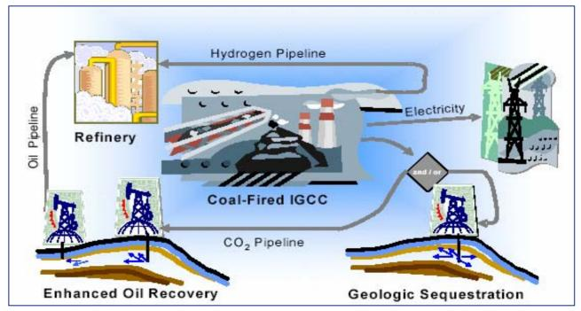
275 MW IGCC with Hydrogen production and 1Mtpa of CO2 sequestered
