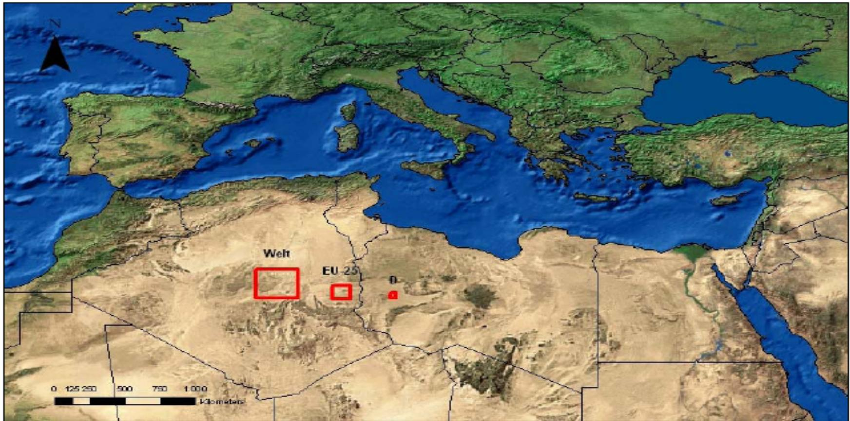
**Fig. 12: Theoretical space requirement to meet the electricity demand of the world, Europe (EU-25) and Germany (Data from DLR, 2005).**
